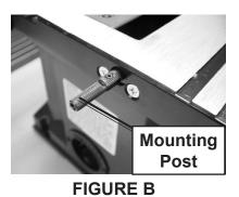
2. Put the Blade Guard Assembly in place over the table. The Support Base (164) of the Guard Assembly attaches to the mounting post shown in **Figure B**, above.
